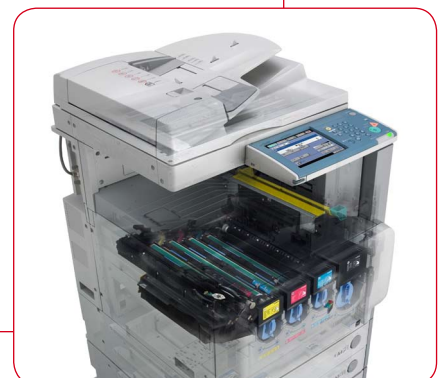
Compact four-drum engine design
